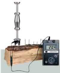
APPLICATION Hydromette HT 85 T unit together with an M 18 ram-in electrode
